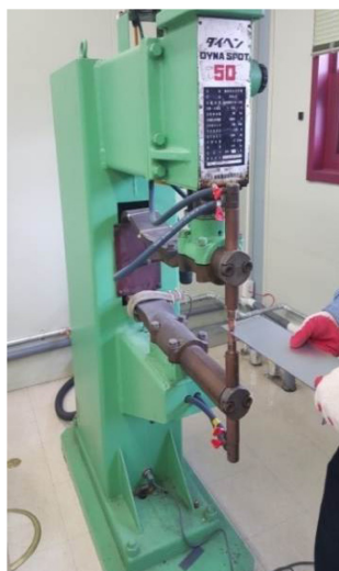
Fig. 1. DYNA spot welding test machine
