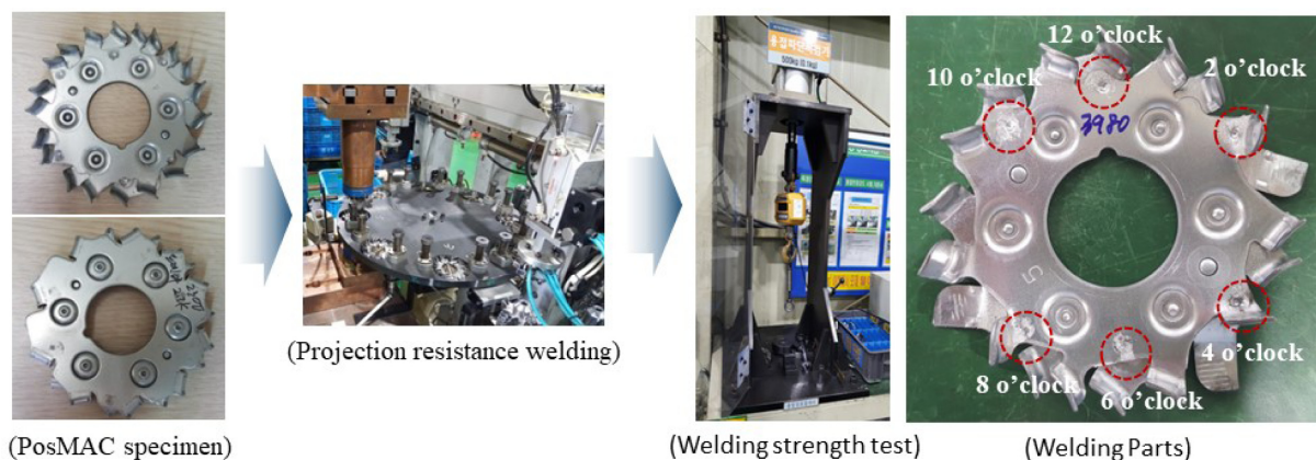
Fig. 8. Projection welding process and measurement of welding strength
