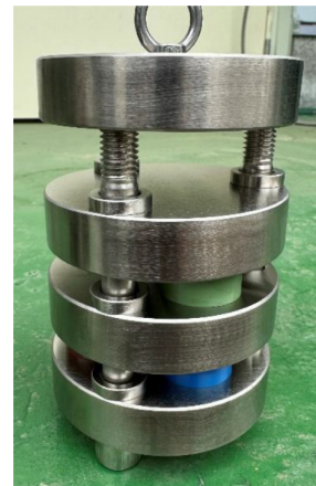
Fig. 4. Compression set jig
