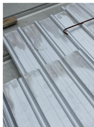
Fig. 1. The photo of black discoloration phenomenon on the surface of aluminum zinc magnesium coating
