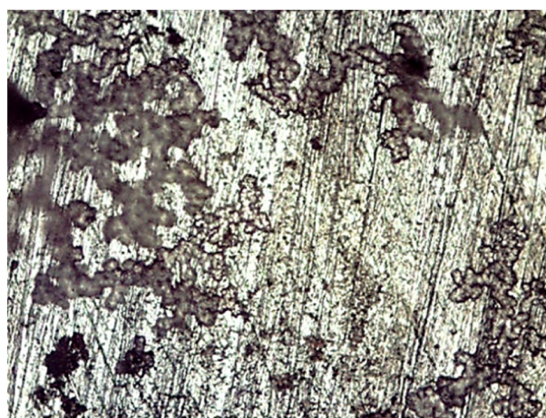
Fig. 13. uncoated substrate's surface were covered with small apatite particles when immersion in SBF
