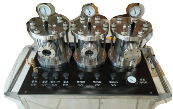
Fig. 1. High pressure chamber for electrochemical experiments
