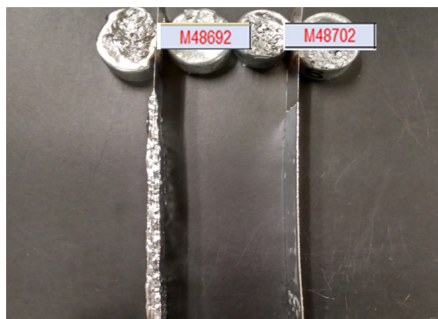
Fig. 5. Zn Coating Buildup (observed in cross-section) on HSLA Steels with Different Si Levels; Open GI Pot, 460 °C, Dip Time: 1.5 hrs
