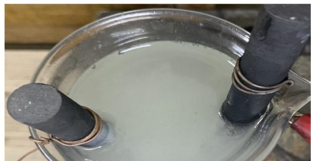
**Fig. 3. The deposition of zinc on the graphite electrode**
