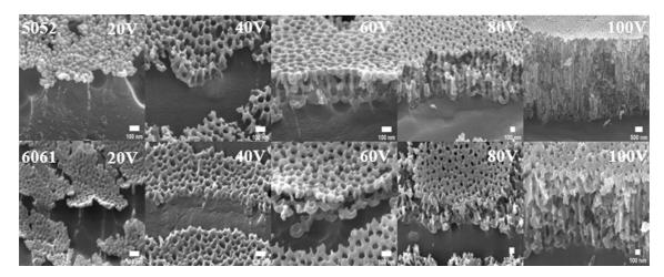
Fig. 4. FE-SEM cross view image by applied voltage for anodization
