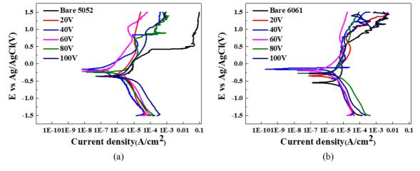
Fig. 8. Potential polarization curve for each applied voltage for anodization: (a) 5052 Aluminum, (b) 6061 Aluminum
