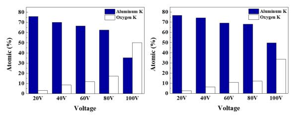
Fig. 2. EDS analysis Comparison of aluminum and oxygen contents by anodization applied voltage: (a) 5052 Aluminum, (b) 6061 Aluminum
