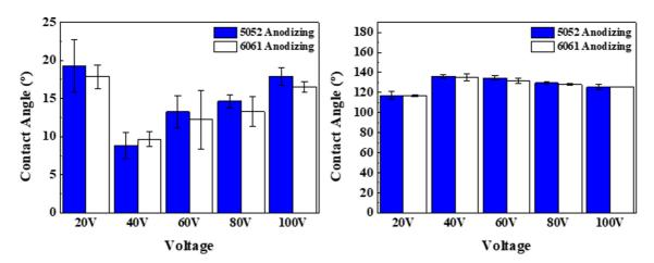
Fig. 7. Comparison of contact angles before and after anodized 5052 and 6061 aluminum coatings
