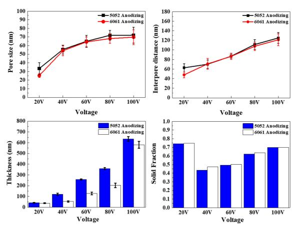
$Fig. \ 5. \ Comparison \ of \ pore \ size, \ interpore \ distance, \ anodization \ film \ thickness \ and \ solid \ fraction \ after \ anodization \ of \ aluminum \ 5052 \ and \ 6062$
