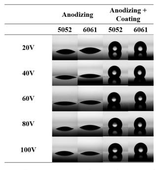
Fig. 6. Contact angle images before and after coating of anodized 5052 and 6061 aluminum
