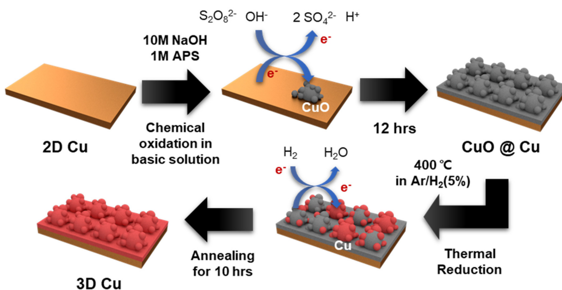
Fig. 1. The fabrication method of 3D Cu current collector using chemical oxidation and thermal reduction, proposed in this work
