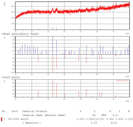
Fig. 7. XRD results of film formed on the failed tube
