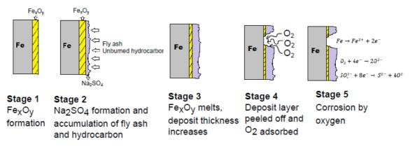
Fig. 8. The schematic diagram of fire side wall tube corrosion
