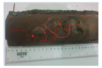
Fig. 2. Photograph of the failed tube after removed from inside boiler.
