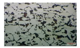
Fig. 3. Optical metallograph of the failed tube
