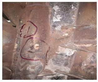
Fig. 1. Photograph of failed tube inside the boiler
