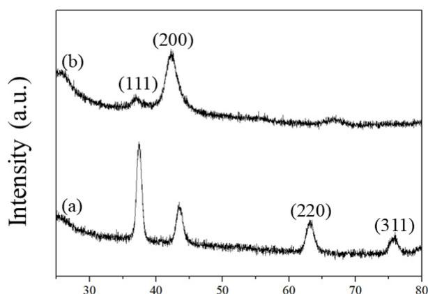
Fig. 1. XRD patterns of the as-prepared CrN films prepared by (a) dcMS, (b) ICPMS
