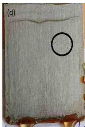
Fig. 18. Optical photograph of 15 % Ch/5 % Gr<sub>2</sub>SiO<sub>2</sub>PVB coatings after 1 week immersion in 0.5 M salt solution.
