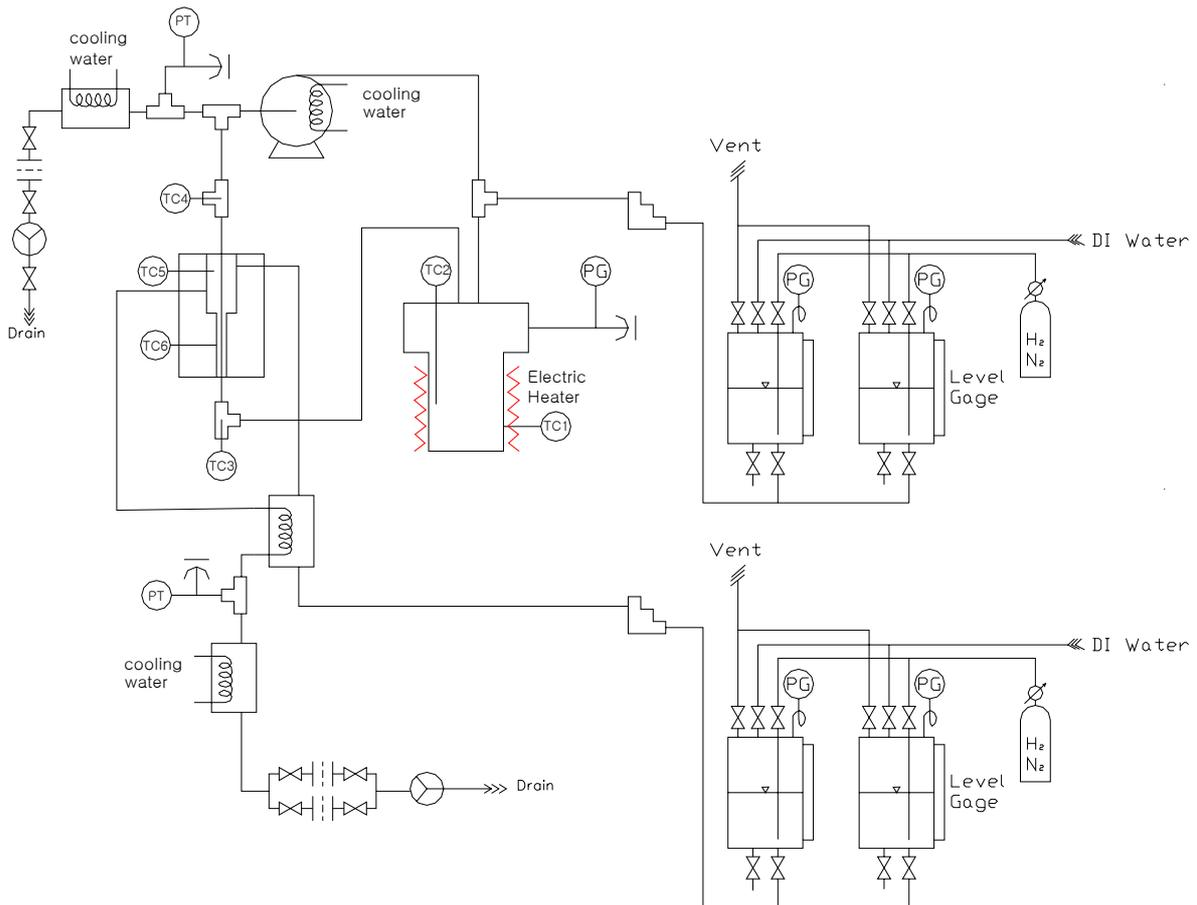
Fig. 3. Schematic of flow accelerated corrosion experimental facility in high temperature aqueous environment.
