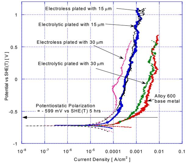
**Fig. 5.** Potentiodynamic polarization curves of Alloy 600 base metal and Ni-plated Alloy 600 in typical PWR water condition.
