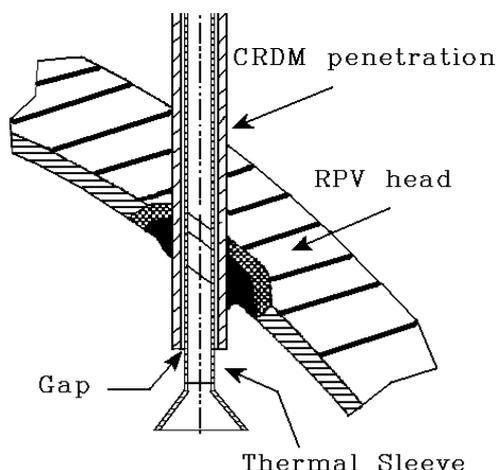
Fig. 1. CRDM nozzle on the reactor pressure vessel head in PWR
