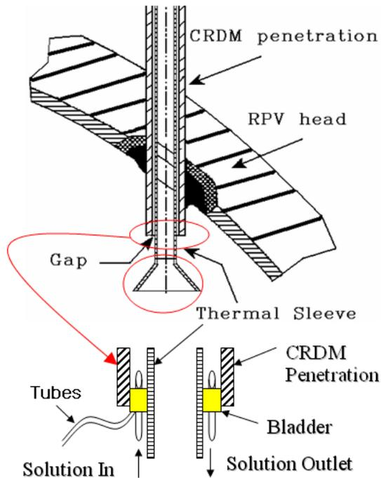
**Fig. 10.** Special end-effector using hydraulic bladder for remote electroless Ni-plating process in CRDM nozzles
