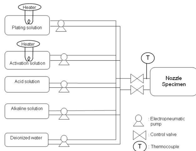
Fig. 7. Schematic of remote electroless nickel plating process.
