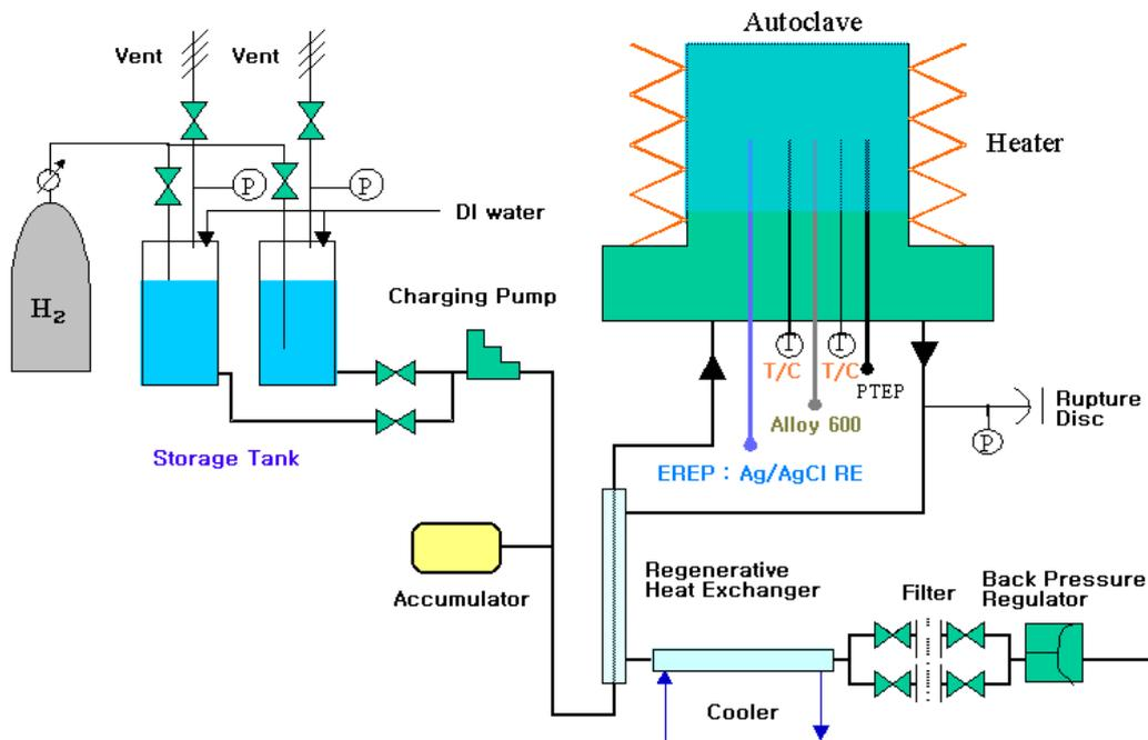
Fig. 2. Schematic of corrosion experimental facility in high temperature aqueous environment.
