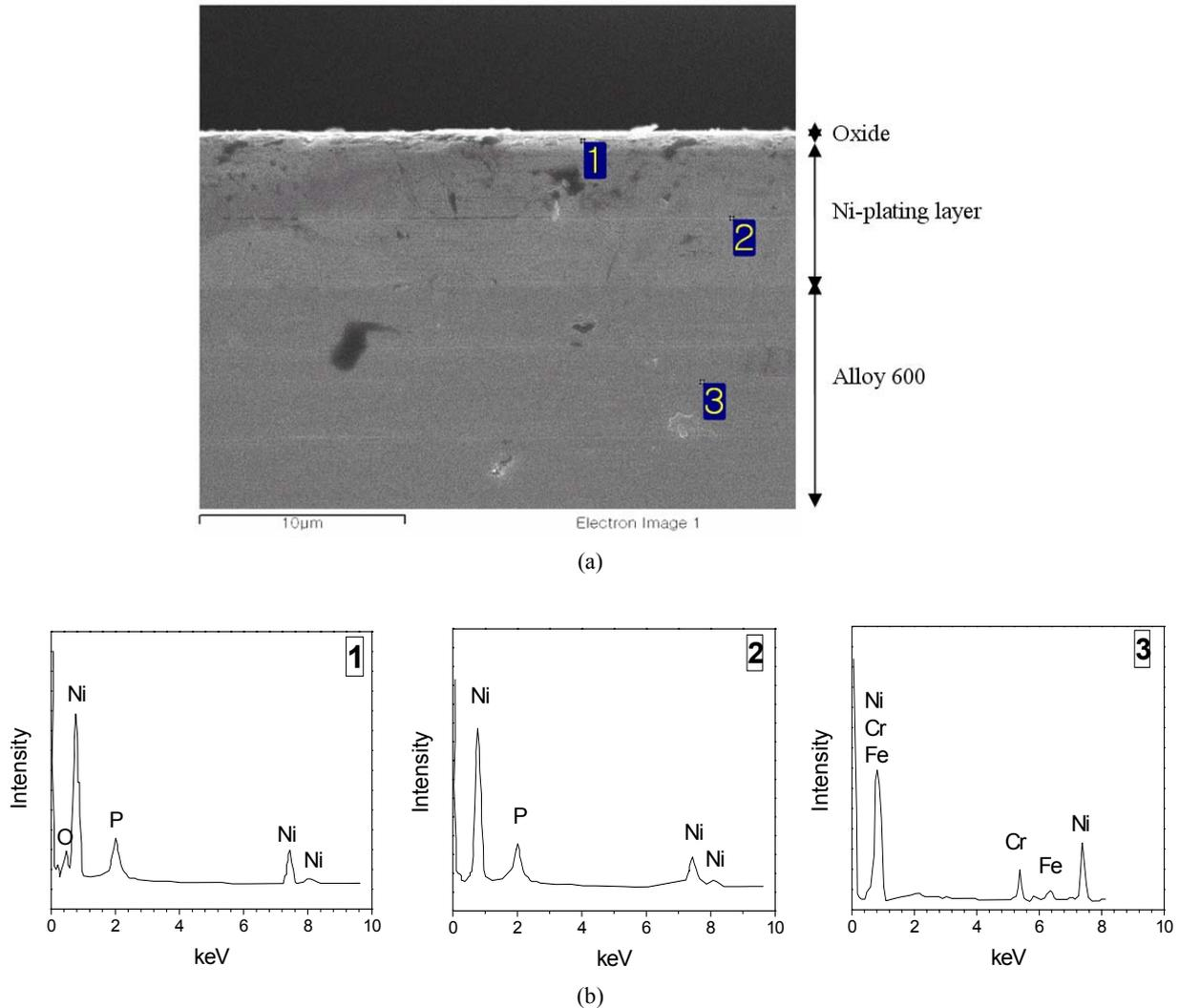
**Fig. 6.** (a) Scanning electron micrograph and (b) EDS measurements of nickel plated Alloy 600 specimen exposed to high temperature, high pressure and high flow-rate water with 250°C, 15 MPa and 2 meter per second for 20 days.
