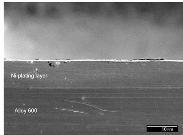
Fig. 9. Scanning electron micrograph of cross section of plate specimen after remote electroless Ni-plating
