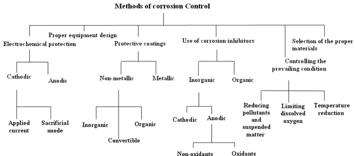
Fig. 3. Methods of Corrosion Control
