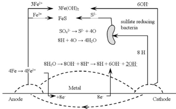
Fig. 2. Chemical reactions ending with ferrous sulfide and ferric hydroxide (corrosion products), where sulfate reducing bacteria play an active role.<sup>7)</sup>
