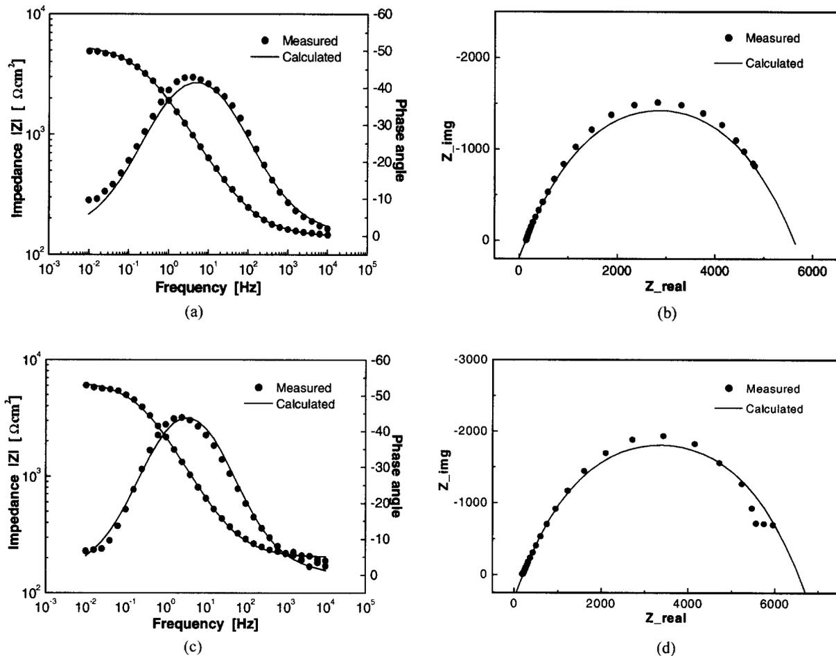
Fig. 3. Simulation for EIS data measured with a thin water film of 0.01M NaCl solution on the specimen surface; (a) and (b) for N1, and (c) and (d) for W2. Bode plot and Phase angle are shown in (a) and (c), while Nyquist plot is shown in (b) and (d)
