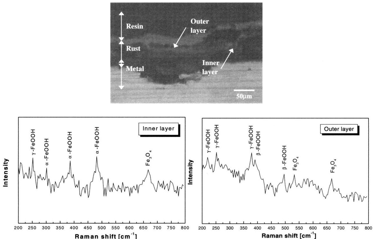
**Fig. 6. Raman spectra of rust layers formed on N1 specimen corroded during 720 cycles**
