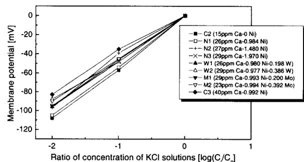
**Fig. 7.** Liquid-junction potentials measured for various rust membranes formed by cyclic corrosion tests
