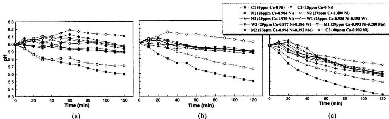
Fig. 2. Change in pH value of thin water film measured for 2 hours at room temperature using a micro-pH electrode; (a) in distilled water, (b) in 0.01M NaCl solution and (c) in 0.1M NaCl
