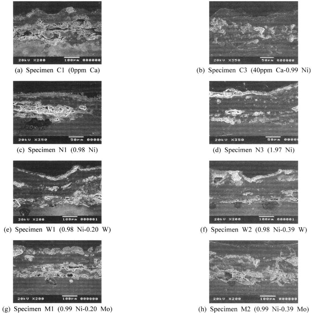
**Fig. 5.** Cross-sectional morphology of rust layers formed on weathering steel after cyclic corrosion tests (720 cycles)
