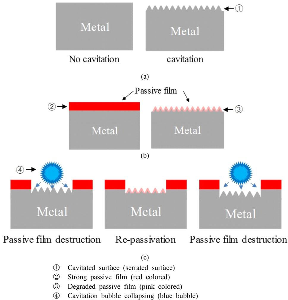
**Fig. 11** New cavitation corrosion mechanism; (a) Increasing surface area after cavitation corrosion, (b) Formation of unstable passive film after cavitation corrosion, (c) Formation of unstable passive film and repeated destruction of passive film during cavitation corrosion.
