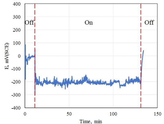
Fig. 6 Effect of cavitation condition on potential change at continuously 2 hours cavitation of additive manufactured CP-Ti in deaerated 3.5% NaCl solution at 25°C.
