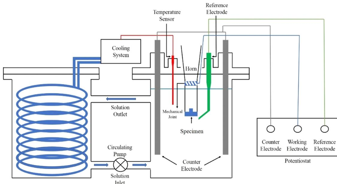
**Fig. 1 Schematic diagram of the cavitation corrosion tester.**
